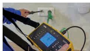
PASS/FAIL LED for viewing the results instantaneously.
