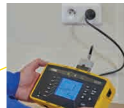
3-pole cable for direct measurements on 2P+E sockets.
